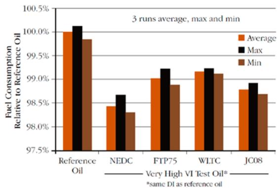
Figure 6: Impact of test cycle on fuel consumption reductions for an engine oil formulation with high viscosity index [23] (Reference oil: VI= 164 (DEXOS 1, ILSAC GF-5), Test oil: VI= 242)
