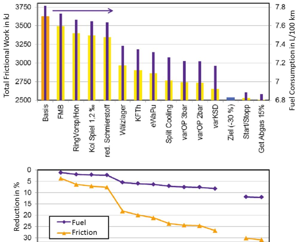
Figure 3: Measures for friction reduction and impact on fuel consumption [14]
