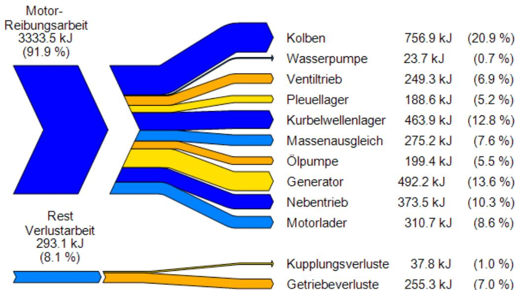
Figure 2: Friction broken-down to the various powertrain aggregates [14]
