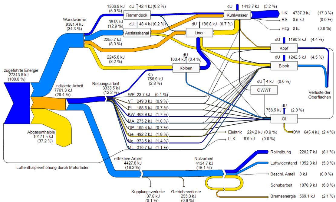
Figure 1: Accumulated energy flows at the end of a NEDC for the basic vehicle (I) [14]
