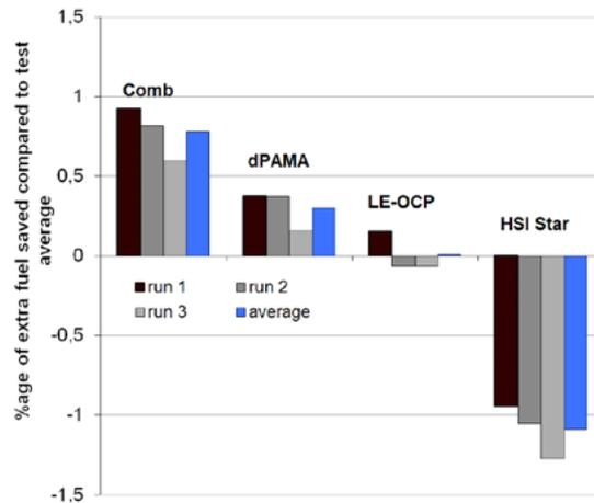
Figure 5: Impact of the molecular structure of a VI-improver on the fuel consumption with engine oils featuring a HTHS von 3.5 mPas (Daimler 350 CGI, NEDC) [22]
