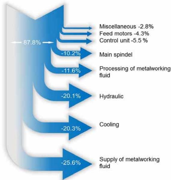
Figure 7: Energy requirements for the individual components of a machine tool [24]
