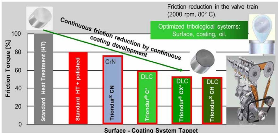
Figure 4: Measures reducing valve train friction (photo: SCHAEFFLER AG)
