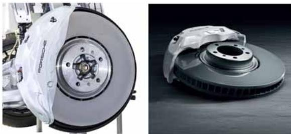
*Figure 11: Porsche Surface Coated Brake (PSCB) with friction surface made of tungsten carbide (PORSCH SE)*
