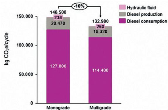
Picture 15: Comparison of total CO<sub>2</sub> emissions [CO<sub>2</sub> e/cycle] for a monograde hydraulic oil (left) and an efficient multigrade oil (right) over 2,000 operating hours [80]
