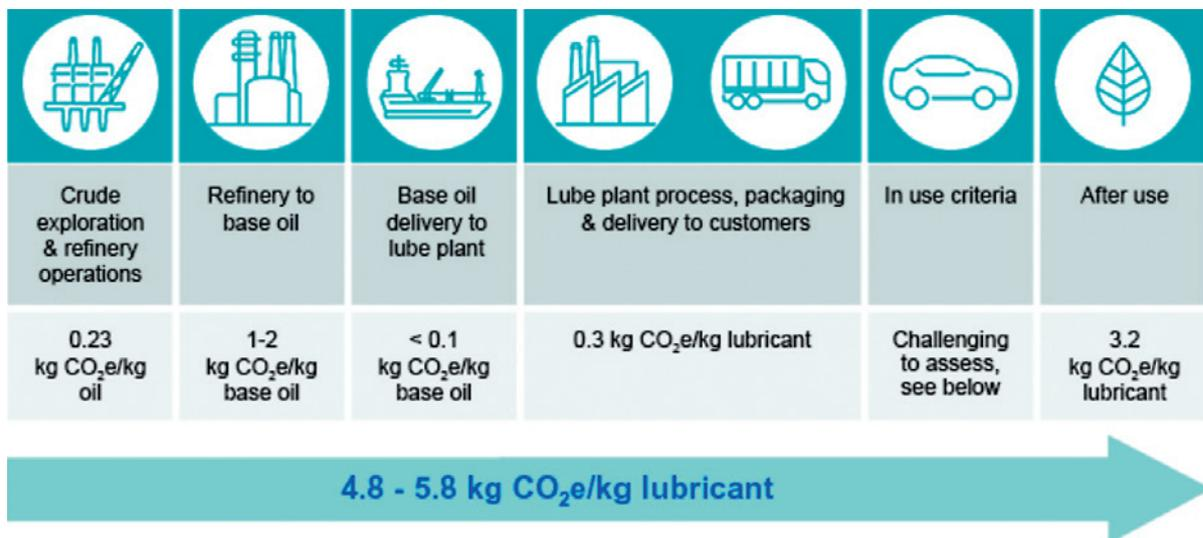
Picture 12: Carbon footprint of fossil-based engine oil production [79]
