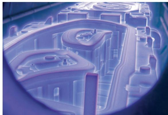
Picture 9: Surface treatment of forming tools by means of BALITHERM® PPD
