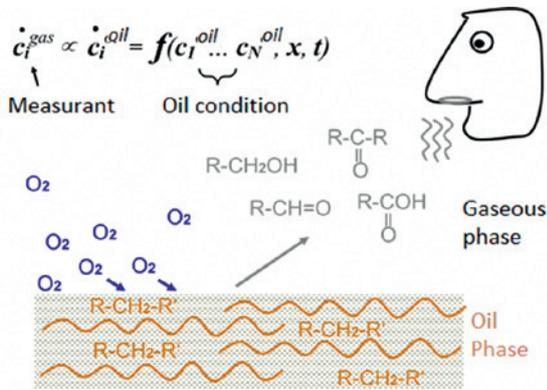
Picture 4: Electronic nose: detection of vaporized ageing products
