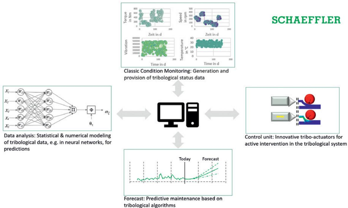
Picture 1: Control loop of a tribotronic system (SCHAEFFLER AG)
