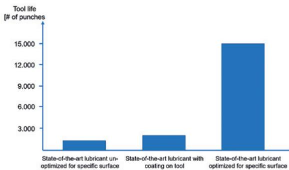
Picture 8: Fine-blanking of stainless steel [FUCHS WISURA]
