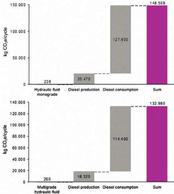
Picture 14: Total CO<sub>2</sub> emissions [CO<sub>2</sub> e/cycle] for a monograde hydraulic oil (top) and an efficient multigrade oil (bottom) [80]
