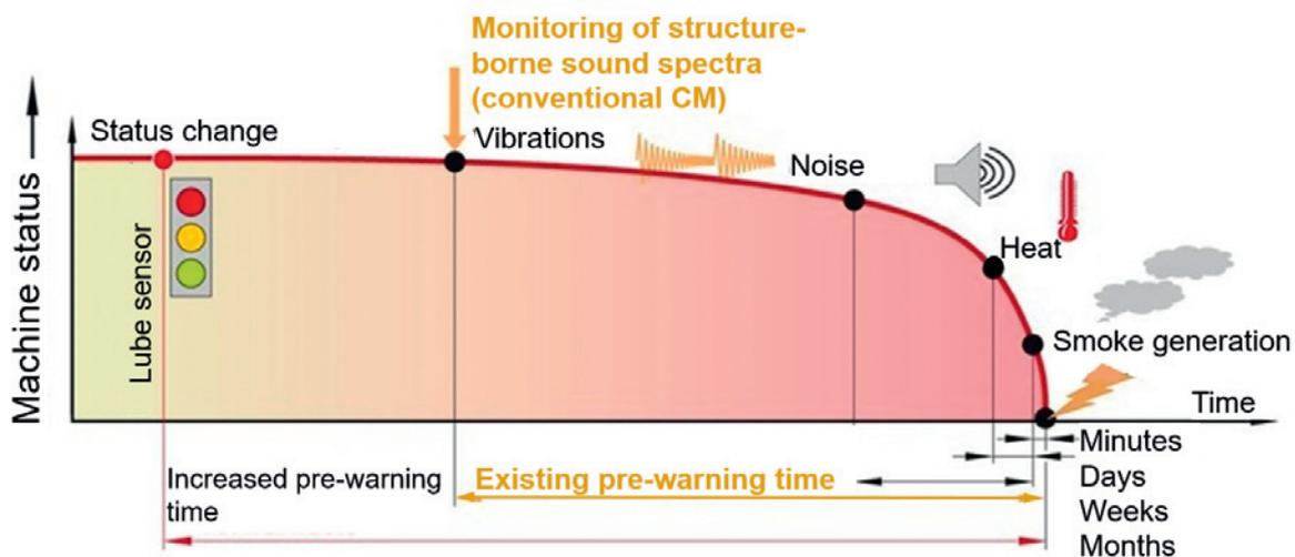
Picture 3: Advance warning periods of methods and events for various machine conditions [43, FAG GreaseCheck]
