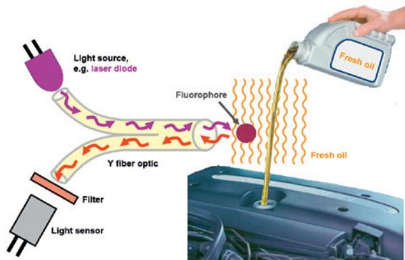
Picture 5: Identification of lubricating oils during the filling process by means of fluorescence analysis
