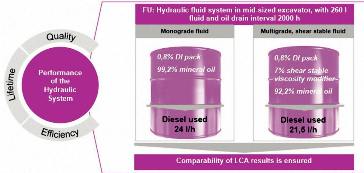
Picture13: Parameter for the life cycle analysis of hydraulic oils in a mid-sized excavator during 2,000 operating hours (EVONIK) [80]
